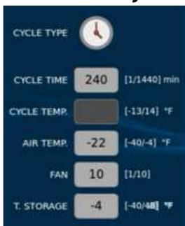
During a Time Cycle (clock icon in the *CYCLE TYPE* tab) the unit will run the cycle pulling down and holding the temperature inside the cavity at the desired temperature set in the “*AIR TEMP.*” tab, for the desired target time set in the “*CYCLE TIME*” tab.
