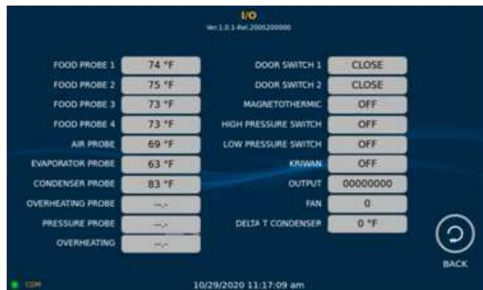
The *Input/Output* menu allow to check all incoming signals, such as temperature sensors, door switch status, the relays status.
