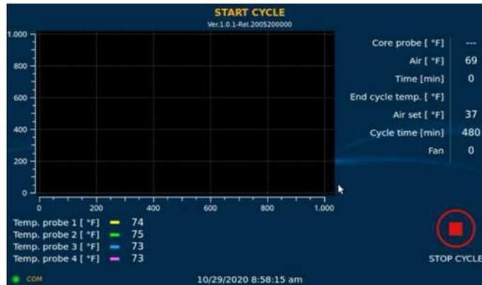
On the right side of the screen instead the hottest core probe value, the cavity temperature, the counting time from the start of the cycle, the end cycle temperature set point, the cavity temperature set point, the cycle time set point and the fan speed are displayed.
